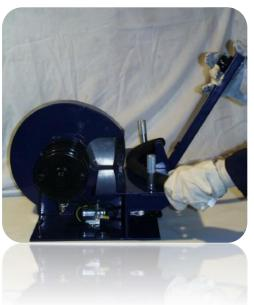
3. Push handle towards blade with a smooth action without forcing the hose onto the blade and let the blade cut through it.
